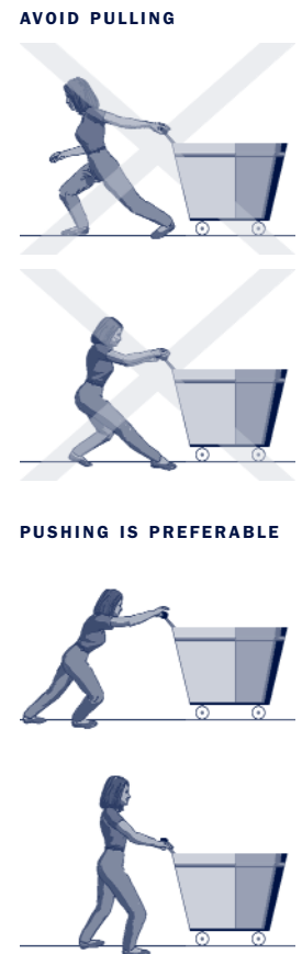
Figure 2. Given the choice between pushing and pulling, a task should be designed for pushing.
